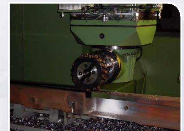
Heavy duty milling head with a powerful 68 kW spindle motor
