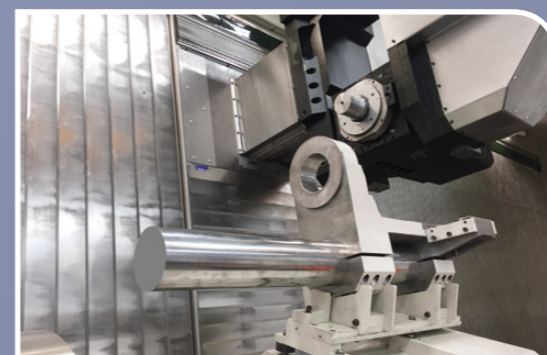
Boring bar holder for milling head with parking position on tailstock
