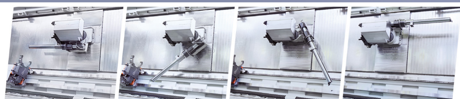
Special boring bar attachment for deep boring operation. The unit is designed for boring bar 120 mm in diameter. The boring bar is mounted on swivel holder that lets the bar be put on parking position without disassembling.
