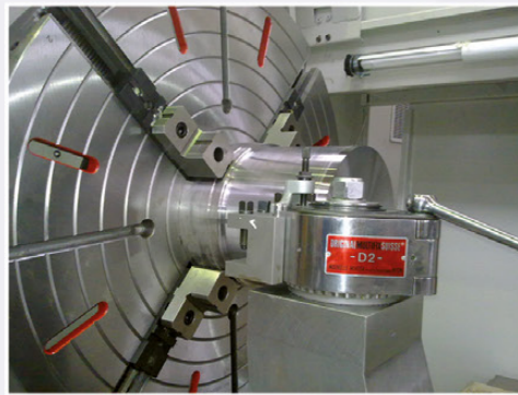
Standard Multifix D toolpost
