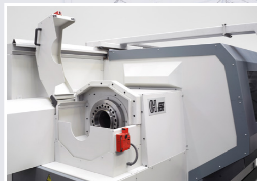
Second spindle nose with complete interlocked covers.
