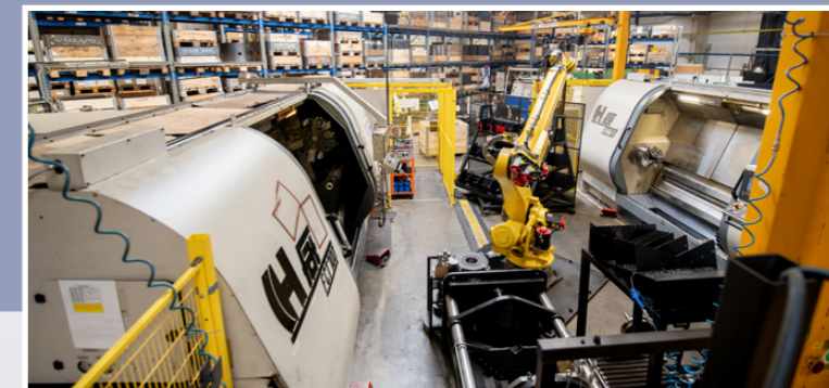
two machines FCT 700 x 2100 with robot integrated together with Fanuc system control
