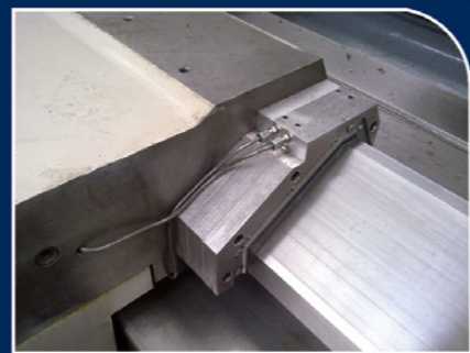
Double scrappers with compressed air for special guide ways security against grinding powder.
