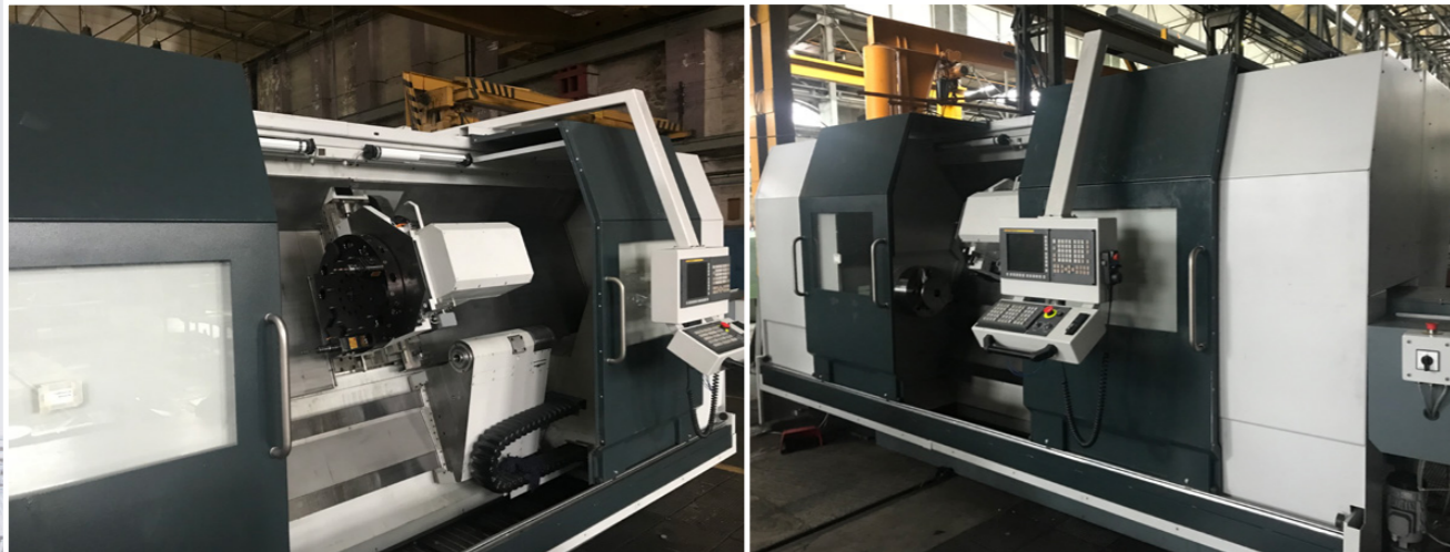
FCT 700 x 1600 with 12 position disc turret with integrated Y-axis
