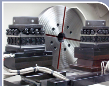
Combination of two 4-positions Sauter head-type turrets
