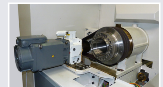
Compact headstock with direct drive and planetary gearbox
