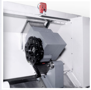
Standard 12 position turret with static tools VDI 30 seats
