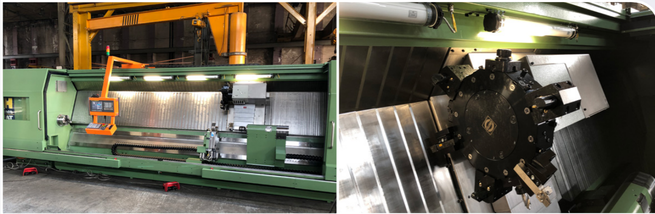
FCT 700 x 5100 with Fanuc OiF, automatic door, hydraulic chuck, self centering steady rest
