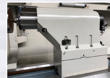
Heavy duty tailstock 280 mm
