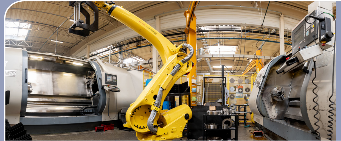
two machines FCT 700 x 2100 with robot integrated together with Fanuc system control
