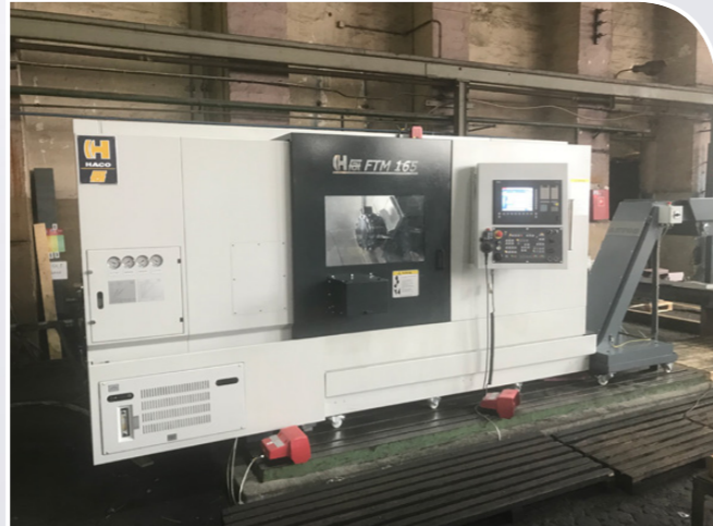
FTM 165 with Y axis turret and subspindle
