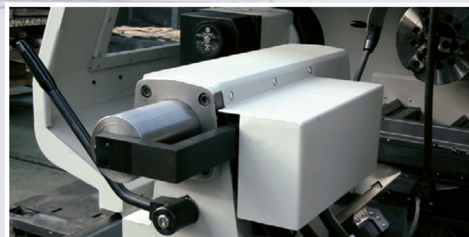
Hydraulic tailstock as an option. Quill diameter 100mm and specially extended neck. Thanks to this solution there is easy access for machining close to the tailstock's centre and high rigidity of total construction.
