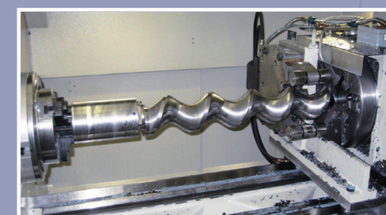
Installation of whirling unit
