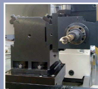
Tooling system mounted on cross-slide T slots
