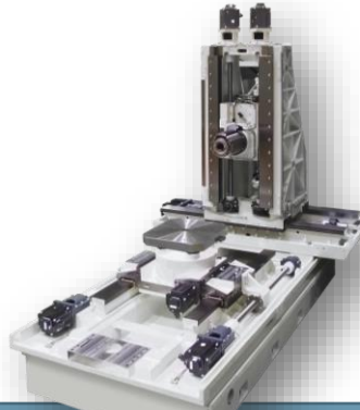
Solid Column Construction
