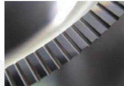
Surface roughness: 0.025 μm Ra
