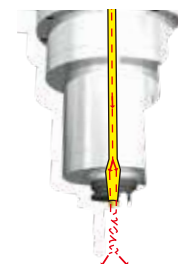
30 bar coolant through spindle
