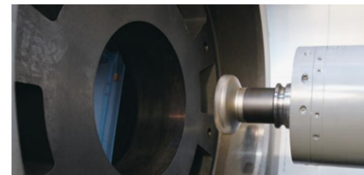
**Large torque 6,000min<sup>-1</sup> spindle** achieving the best performance in its class **Option** FH1000SX FH1250SX
