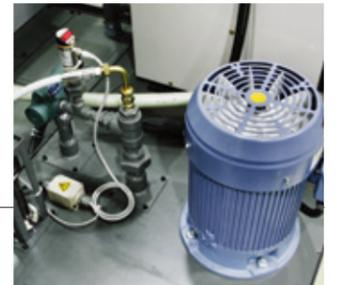
Spindle-through coolant 3MPa
