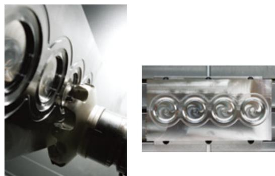
**Large torque 15,000min<sup>-1</sup> spindle** Multi-use spindle that achieves 530N·m in low speed ranges, even with a high-speed spindle **Option** FH1000SX FH1250SX
