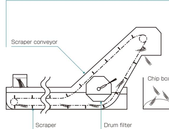
**Option Two-tiered coolant supply unit with chip conveyor**
