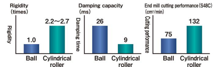
Because of JTEKT's assembling technology which allows for strict mounting face accuracies, the rigid cylindrical roller slide offers the best rapid feed rate and acceleration in it's class.
