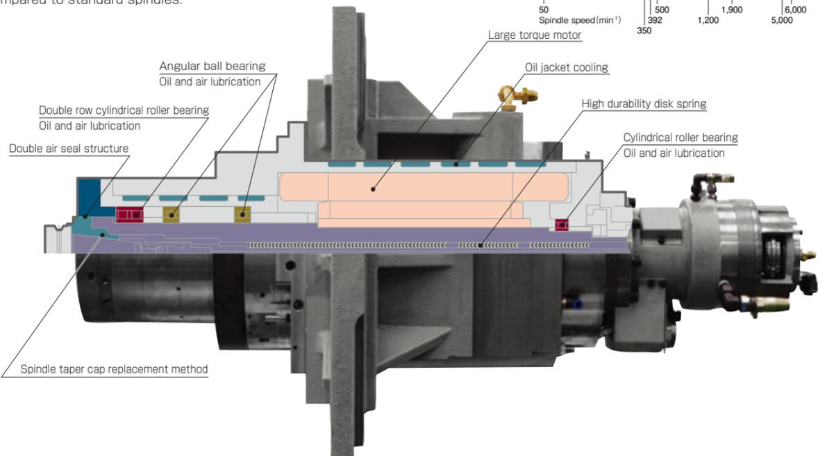
**Best cutting performance in its class with a 1,009N·m large torque spindle**
