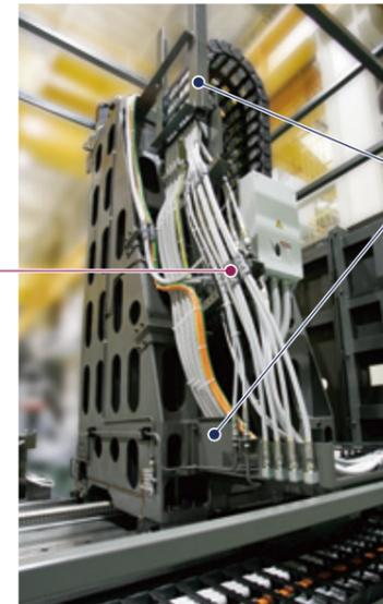
Piping and wiring cables are tied to reduce sagging - a measure in response to higher speeds and acceleration.
