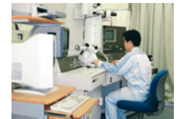
Using a transmission electron microscope to survey metal structure
